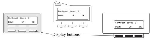
Some display buttons, such as TRANSFR and ALL, are shortcuts that are only available on a two-line display. Other display buttons, such as OK and SHOW, perform a function necessary to proceed. Table 3 shows display button functions and dial pad buttons on a one-line display telephone. See "Substitutes for buttons on a one-line display telephone" on page 26.
