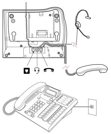
Figure 3 shows the T7316 and stand wall mounting procedure. See "Mounting a T7316 telephone with a stand on the wall" on page 22.
