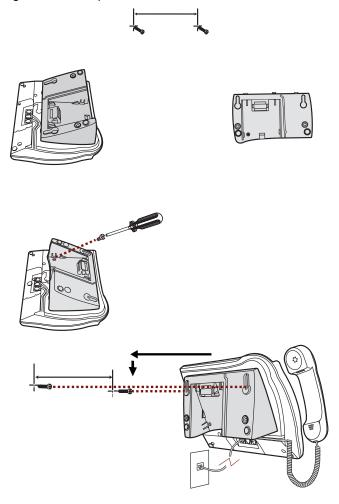
Figure 4 shows the T7316 without a stand wall mounting procedure. See "Mounting a T7316 telephone without a stand on the wall" on page 23.
